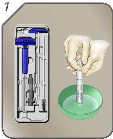
Heparin Flush: rinse all kit components with heparin (2,000 Units/ml)
